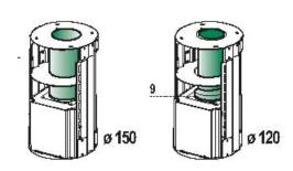
When installing the ducted version, connect the hood to the chimney using either a flexible or rigid pipe Ø 150 or 120 mm, the choice of which is left to the installer.
