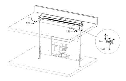
• Tighten the screws 12c and 12b completely.
