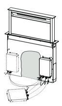
⚠ Warning..: Do not install the product in such a way that the wiring box is in contact with the floor.
